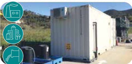
Containerized pilot plant for brackish water applications (UF)
