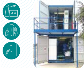
Containerized pilot plant for brackish water applications (UF)
