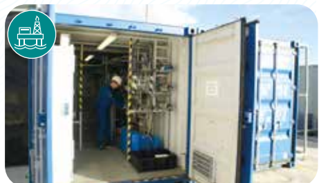
Containerized pilot plant for Oilfield application (UF + NF/RO)
