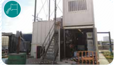
Containerized pilot plant for Ion exchange applications (IX)
